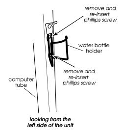
Figure 10 - Install Water Bottle Holder
